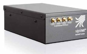
The MultiAMP Combiner increases the quality of sending and receiving 3G/UMTS mobile radio signals. The device is interconnected between a maximum of four UMTS/HSPA+ modules in Viprinet Multichannel VPN Routers and one mobile radio antenna, and is able to compensate for distances of up to 25m between router and antenna without any signal loss.
