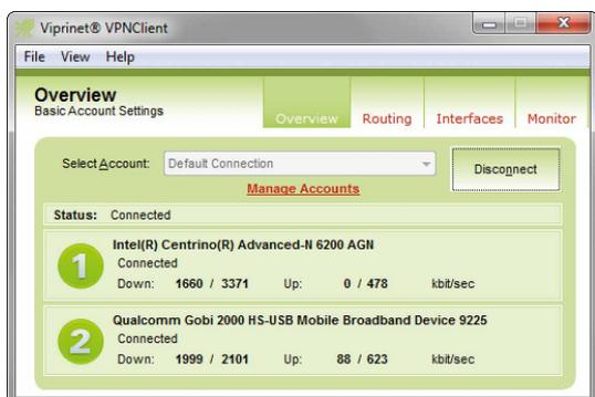
Viprinet’s VPN Client enables bonding two Internet connections without any further hardware, e.g. one Wi-Fi link and one 3G mobile phone connection. At the same time, an SSL-encrypted VPN tunnel is established. The user interface can be easily operated, and gives an extensive overview over the utilization and performance of the connections bonded.
