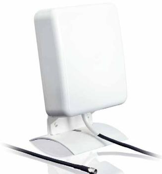
3G/UMTS signals are often poor in buildings. Here, this outdoor antenna helps. In its weather-resistant and stable housing, an ultra-wideband receiver is installed which gains up to 11 dBi. The antenna is suitable for simple wall or pole mounting; it must be directed at the transmission tower of the respective mobile service provider employed.
