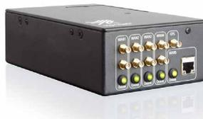
The model series 51X was also designed for ultra-mobile usage scenarios, but comes with more complex inner workings. Here, four integrated LTE/DC-HSPA+/EDGE/GPS modems ensure the best possible bandwidth from all available mobile phone connections.
