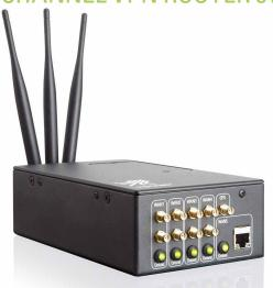
The Multichannel VPN Router 512 stands out due to its robust and power saving layout. It comes with 12 antennas (8x LTE, 3x WiFi and 1x GPS); the eight SMA connectors also allow for the alternative use of external antennas. With that, it meets all demands made to a fast and highly available Internet connection for many intended uses.
