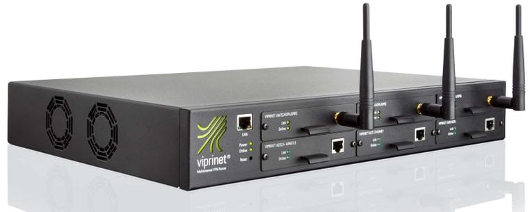
This 19"-sized router allows the bonding of up to six different WAN lines into a single, high-performance virtual link. Its maximum bonding capacity is 125 MBit/s. Thus, the router will offer enough bandwidth for establishing company networks of different sizes. By adding or substituting single hot plug modems, the network structure can be individually adapted to changing requirements.
