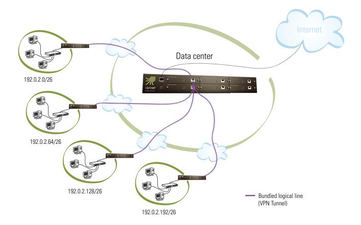
Both networks reach each other using the peer located at the Internet backbone. Packets going out from network A and directed to network B or vice versa are directly being transferred inside the router from VPN tunnel A to VPN tunnel B. Packets to the Internet use the public IP address from that network as source address. Both networks are reachable from the Internet.
