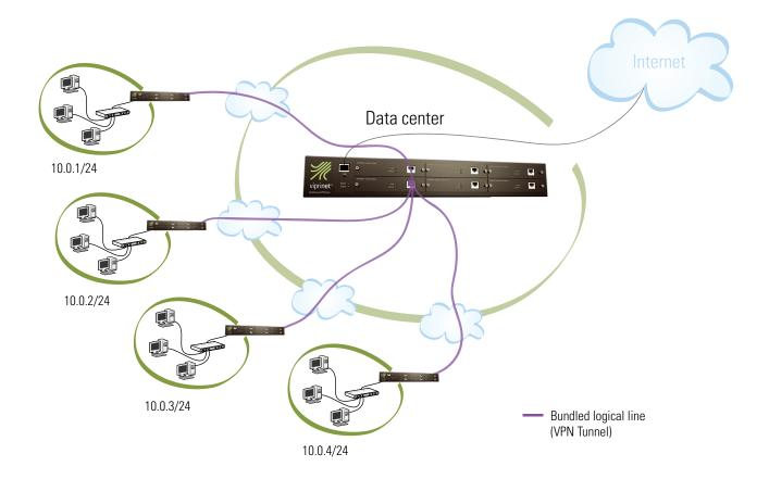
Once again both networks reach each other using the peer located at the Internet backbone – it's not a problem that their private addresses cannot be routed in the Internet, since the packets are transferred over a VPN tunnel. Packets from network A to network B or vice versa are directly transferred from VPN tunnel A to VPN tunnel B inside the router. Packets towards the Internet get assigned a new, public source address via NAT at the peer.
