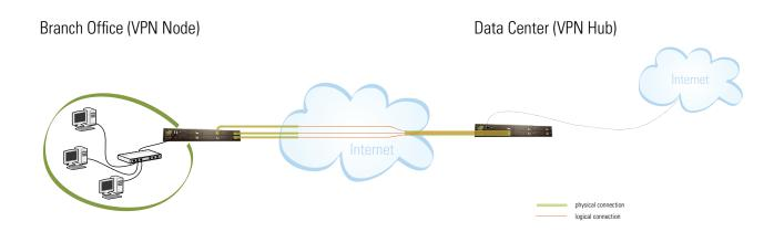
From this it follows that the Hub used should be well reachable from all physical line providers. We recommend setting this Hub up in a data center directly connected to a backbone provider or directly at an ISP exchange point. Alternatively you can operate the peer in a "branch office networking" use case, provided that the branch office is equipped with a reliable broadband Internet connection.
