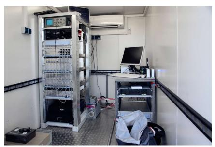
WERA radar system with receivers, process computers and the Multichannel VPN Router (rear right)
