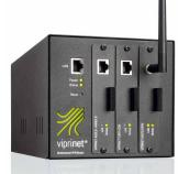
The Multichannel VPN Router 300 is the perfect solution to connect small offices to the Internet or a corporate VPN via up to three Internet connections. Thanks to its three module slots, the device is suited for all current and future broadband technologies, and can be utilized very flexibly.
