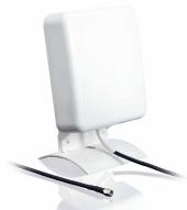
3G/UMTS signals are often poor in buildings. Here, this outdoor antenna helps. In its weather-resistant and stable housing, an ultra-wideband receiver is installed which gains up to 11 dBi. The antenna is suitable for simple wall or pole mounting; it must be directed at the transmission tower of the respective mobile service provider employed.
