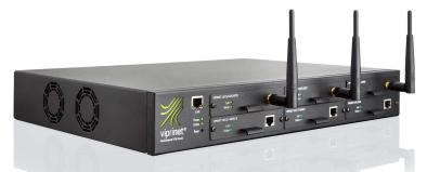
This 19"-sized router allows the bonding of up to six different WAN lines into a single, high-performance virtual link. Its maximum bonding capacity is 125 MBit/s. By adding or substituting single hot plug modems, the network structure can be individually adapted to changing requirements. Thus, it offers long-term security of investment for medium sized and large businesses.
