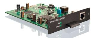
This integrated modem hot plug module is to be directly connected to the ADSL/Phone splitter box — an external ADSL modem is no longer required. As the router is able to directly control the chipset of the integrated modem, it is able to achieve optimized performance — even fully utilized lines stay low in latency, suitable for VoIP applications. This modem module supports ADSL with Annex-A speeds of up to 25 Mbit/s in the downstream direction.
